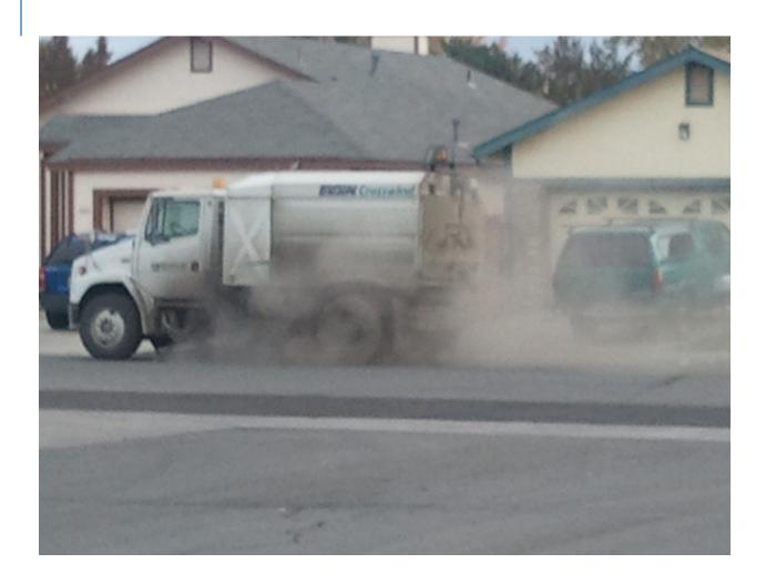
Sweepers water is not on. Leaving a cloud of dust 11/11/2011.
